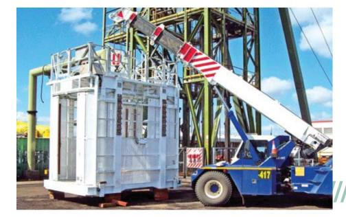
The 40 man Dolly Car is uniquely innovative due to its increased capacity which allows improved efficiency in the transportation of men underground and versatility to also couple with rail mounted vehicles for materials transportation. Passenger safety, comfort and ease of maintenance are paramount in this design.
